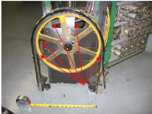
Photo #30 – Electro Mechanical Selector tape sheave
